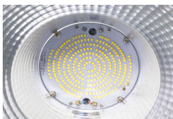
3030/3535 SMD LED, CREE XBD/XPE/XPE supportable
